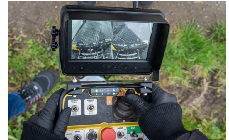
No work at height: remote control from ground level
