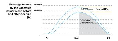
The sunlight reflection effect by dirt decreases the absorption of solar energy on the photovoltaic cells
